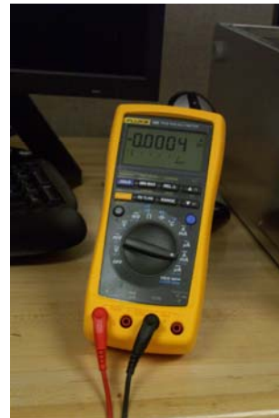
Figure 3. Fluke 189 Digital Multimeter [Created by Richard David McWhorter, III.]
