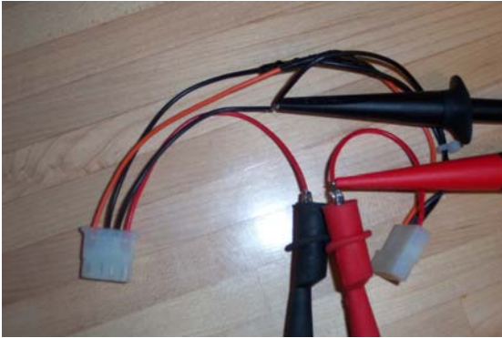
Figure 6. Power consumption test setup for 5V line. The red wire is the positive 5V lead, and is placed in series with the ammeter. The leads exiting the bottom of the picture are attached to the ammeter. The black wires are ground. The voltmeter, whose cords exit the picture to the right, is placed in parallel with the 5V line and ground. [Created by Richard David McWhorter, III.]
