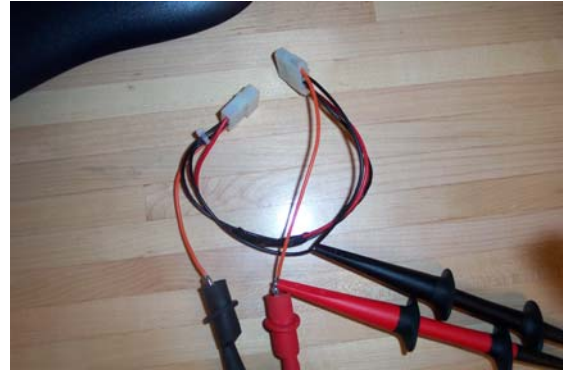
Figure 7. Power consumption test setup for 12V line. The orange wire is the positive 12V lead, and is placed in series with the ammeter. The leads exiting the bottom of the picture are attached to the ammeter. The black wires are ground. The voltmeter, whose cords exit the picture to the right, is placed in parallel with the 12V line and ground. [Created by Richard David McWhorter, III.]
